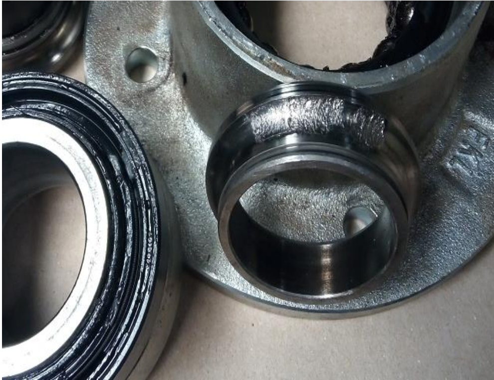
Damage on the inner ring
