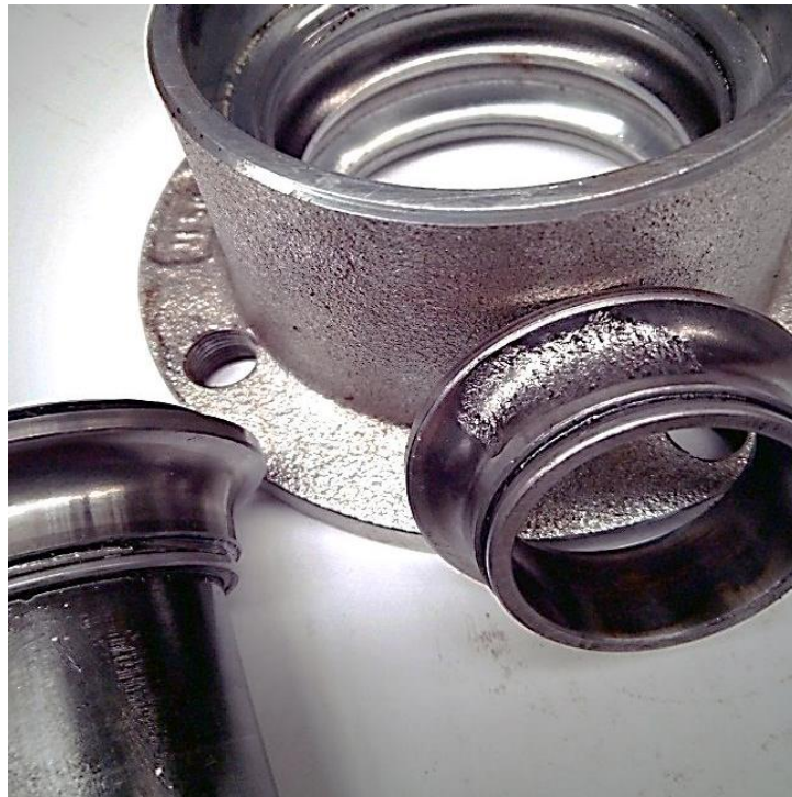
Damage on inner ring
