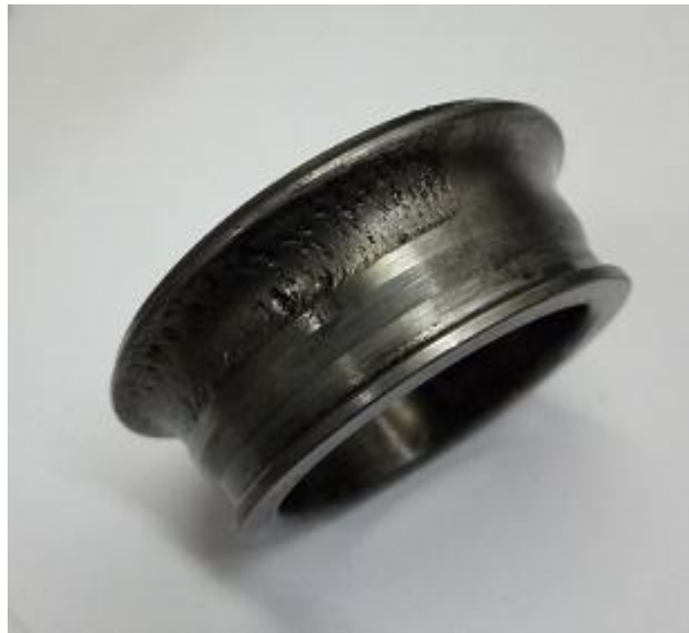
One of two inner rings is damaged
